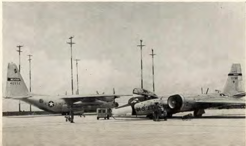
Two of AWS' newest aircraft, the RB-57F of the 58 WRS, Kirtland AFB, N.Mex., and a new WC-130E belonging to the 54 WRS. The WC-130 has been specially modified for weather reconnaissance work to include penetration of tropical depressions, storms and typhoons. The RB-57 is a high-altitude aircraft designed for atmospheric sampling operations.
